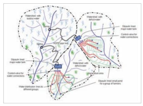
Conceptual diagram of Spring Water-Harvesting (Inter Watershed Water Transfer)
