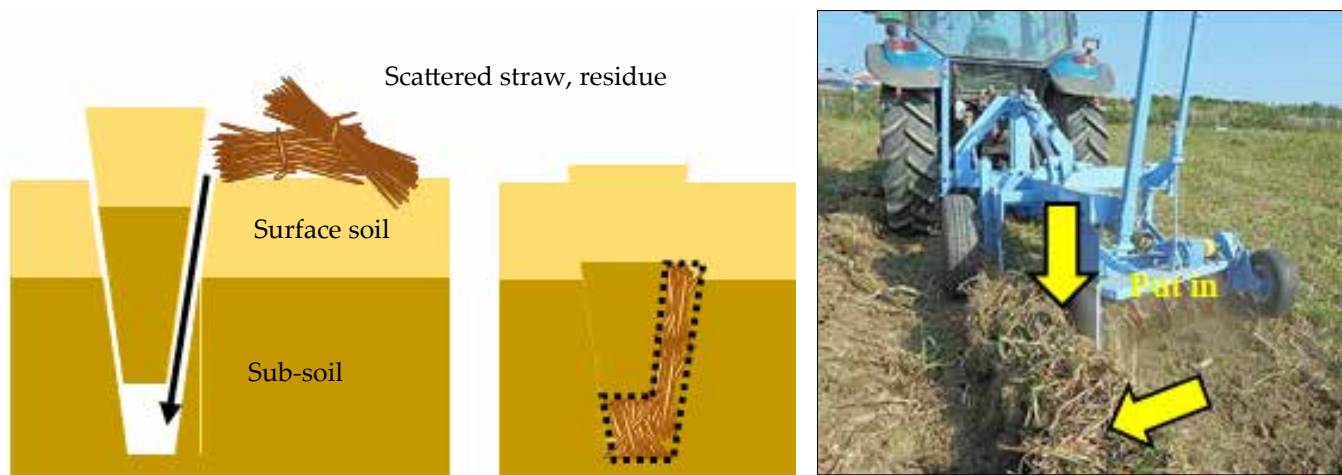
Mechanism of cut-soiler operation for preferential shallow sub-surface drainage construction
