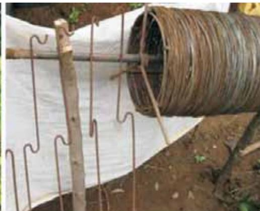
A View of Rolling & Stretching Device
