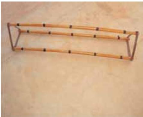
A view of portable simple SRI marker
