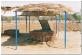
A low-cost passive cool chamber has been developed by the CAZRI, Jodhpur to preserve vegetables for short duration. Conventional methods of refrigeration are costly and not possible due to non-availability of electric power in villages. The chamber can preserve 30–50 kg vegetables.
