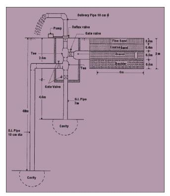
A skimming-cum-recharge structure for extraction of fresh water overlaying saline ground water has been designed at down stream location at Jagsi in Jind district.
