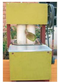
Crushing rollers are designed so that only gel is extracted
