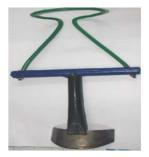
Banana-comb cutter facilitates cutting and separation of banana comb with minimum damage
