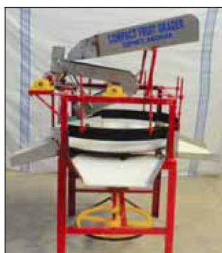
Compact fruit grader developed at CIPHET Ludhiana/Abohar
