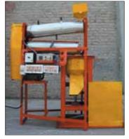
unit, *makhana* is heated at 200 to 300°C, and then conveyed to decortication /popping unit. The popping unit consists of a casing and an impeller assembly with a hard impact surface. When hot nuts strike the impact surface, shells get broken, and due to sudden drop in the pressure, kernels pop-up. The design of this machine has been licensed to M/s Jwala Engineering and Consultancy Ltd, Ambala, for mass manufacturing and marketing.
