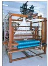
to run large shuttle (up to  $40 \text{cm} \times 5 \text{cm}$ ) that can accommodate larger (up to 18 cm length) pirn. The yarn content in the pirn increased to 24 g (almost 400% higher) as against 6.5 g used in the traditional
