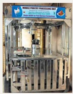
The stainless steel unit weighing 500 kg is of  $2,410 \, \text{mm} \times 1,345 \, \text{mm} \times 2,058 \, \text{mm}$ , and costs approximately `5.50 lakh (2012-13). Its capacity is 35-40 birds per hour. It consists of two water tanks, bleeding cones and troughs, a scalding tank, a de-feathering machine, a carcass washing unit, a teflon board for cutting carcasses, an insulation box, crates for holding 50 line birds and work area for preparation of value-added products.
