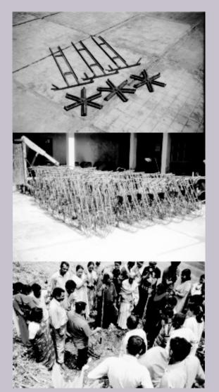
Development of fixtures for manufacture of wheel hoe handle and wheel (top); batch production of wheel hoe seed drill (middle), demonstration of improved implement at farmer's field (bottom)
