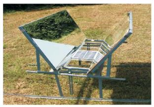
Concentrator for solar photovoltaic panel
