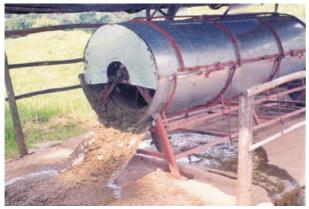
Biogas plant slurry dewatering machine
