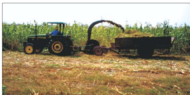
Forage harvester-cum-chopper. Field trials were conducted for pearl millet and maize
