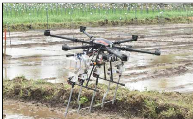
Drone-mounted seed and fertilizer spreader in rice
