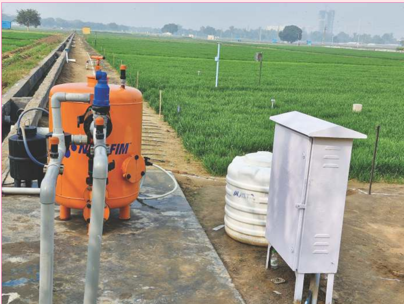
Sub-surface drip fertigation system
