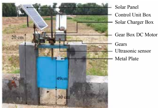
Automated surface irrigation system
