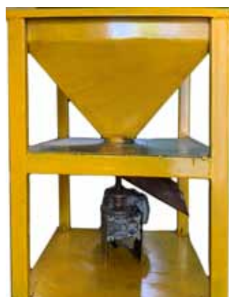
Rotating Orifice Feeding System for Makhana popping machine
