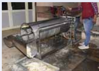
Peeling machine for medicinal root crops
