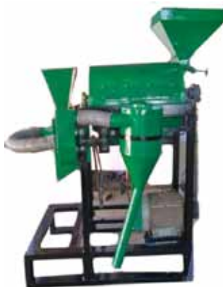
Small Millets Dehuller (Abrasive type)
