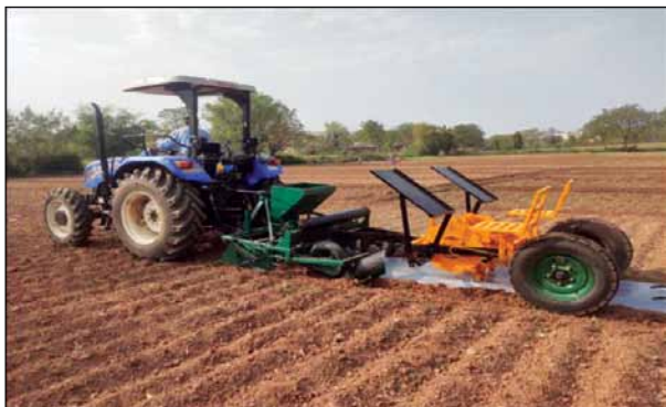
Raised bed mulching and drip laying machine
