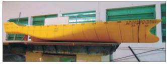
Model of the 19.75 m multi purpose fishing vessel used for testing at IIT, Chennai.
