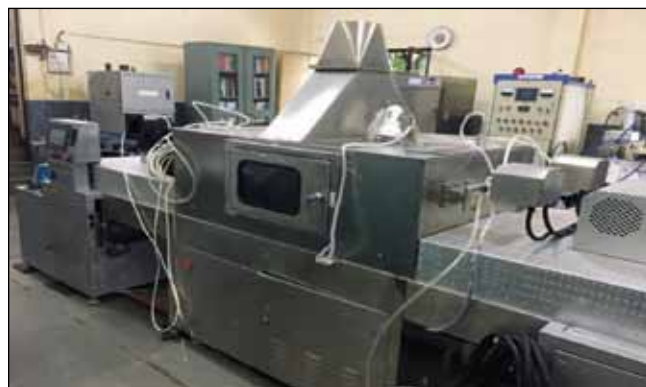
Continuous microwave disinfestation system for food grains
