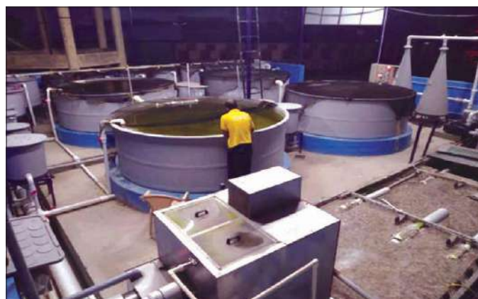
A pilot scale rainbow trout Recirculating Aquaculture System
