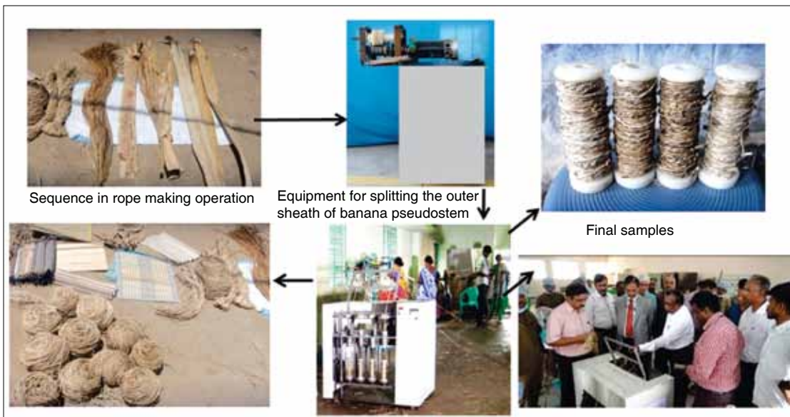
Flow chart of mechanization package for rope making from outer sheath of banana pseudo stem
