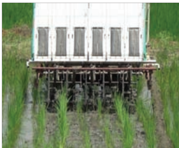
Paddy weeder attachment to six-row self-propelled paddy transplanter
